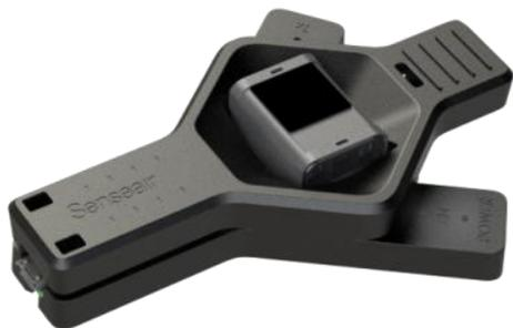
By connecting the Senseair Sunrise Evaluation Kit to the PC where Senseair standard software [UIP5](#) installed, the Senseair Sunrise sensor can be easily evaluated before start designing the host system.
