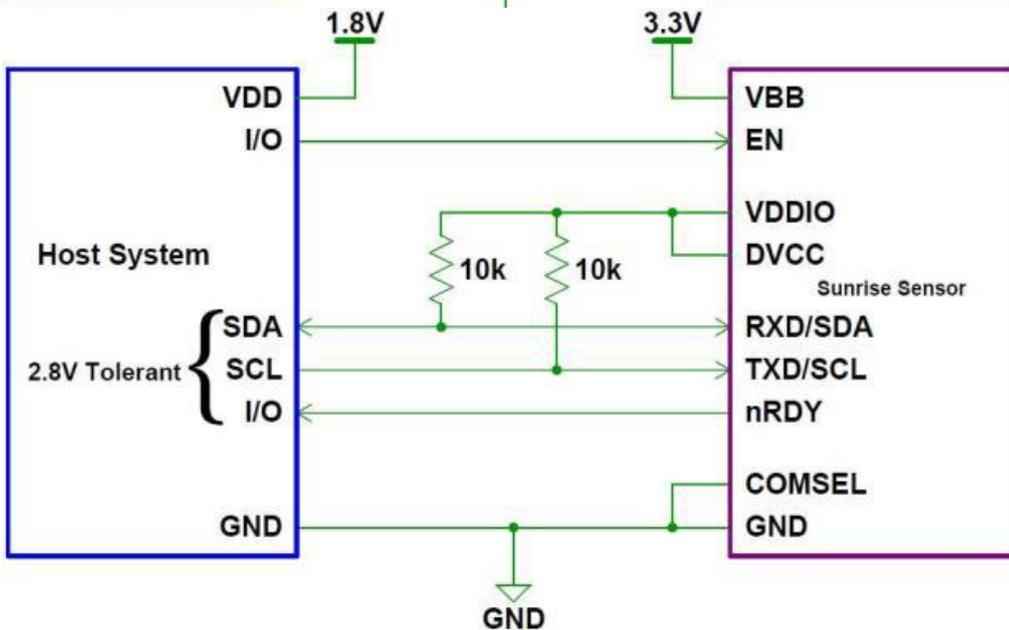
1.8V powered host and low-power I2C integration example for continuous-mode or single-mode integration. Host controls and toggles EN-pin and Sunrise VDDIO is powered from a 2.8V tolerant host source.
