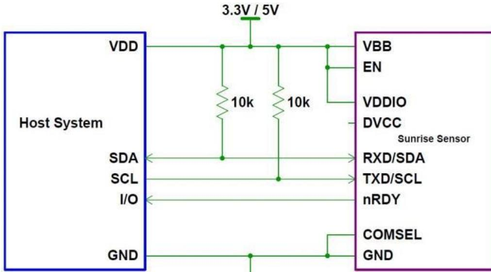
Example I2C integration strictly for continuous-mode operation of Sunrise, as EN-pin can't be toggled and VDDIO is driven by VBB. This will consume more power.
