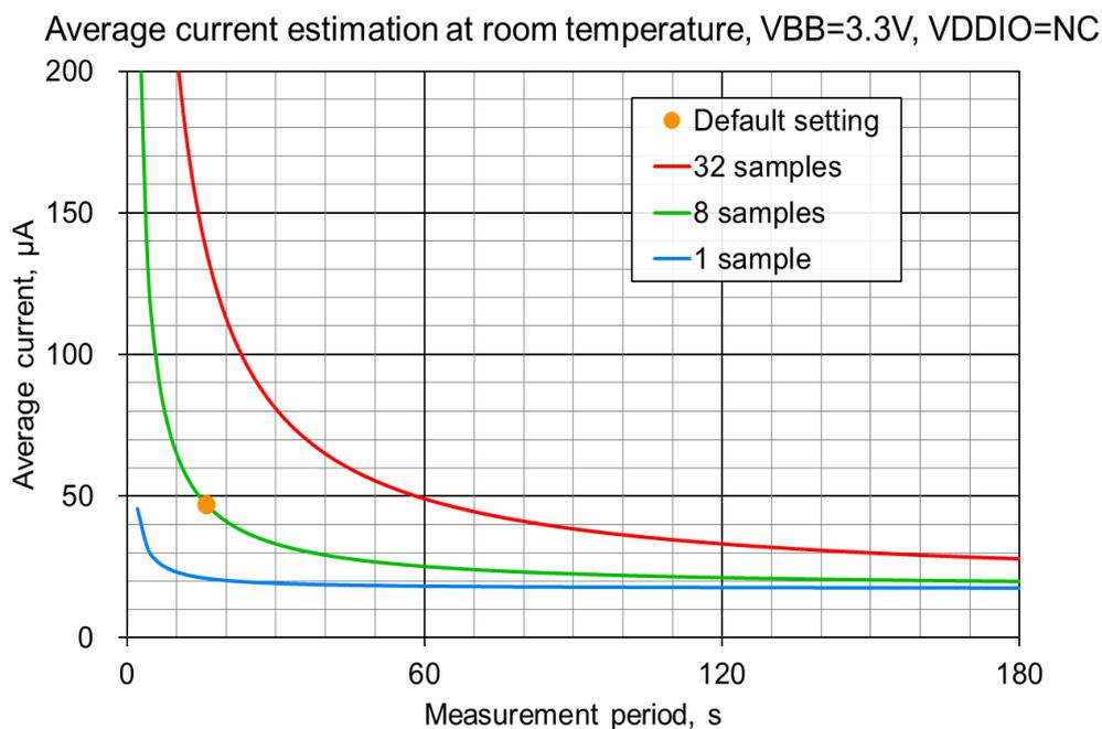
Power consumption diagram @ single measurement mode
