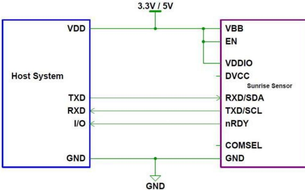
Modbus serial-line over UART. Integration strictly for continuous-mode operation of Sunrise, as EN-pin can't be toggled and VDDIO are driven by VBB. This will also consume more power.
