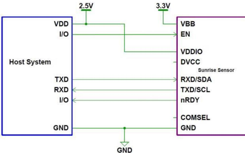
2.5V powered host and low-power integration example for continuous-mode or single-mode integration. Host controls and toggles EN-pin and powers VDDIO externally from Sunrise's VBB.
