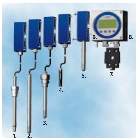
Figure 1. HMT360 series transmitters comprise four detachable parts – (6) an electronics unit, (7) a mounting plate, (8) a transmitter base unit, and a wide selection of probes, which are pictured from the left: (1) HMP368, (2) HMP365, (3) HMP364, (4) HMP363 and (5) HMP361.
