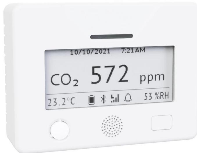
Aura-CO2 embeds the eLichens Foxberry CO2 gas sensor, a cutting-edge dual-channel NDIR (Non-dispersive Infrared) gas sensor integrated in a small and compact form factor. It is based on eLichens' patented technology including a proprietary IR micro-source, patented optical design and advanced signal processing algorithms. Using the auto calibrated Foxberry gas sensor ultra-low power mode, Aura-CO2 reaches more than 5 years on battery without recharging, maintenance or calibration.
