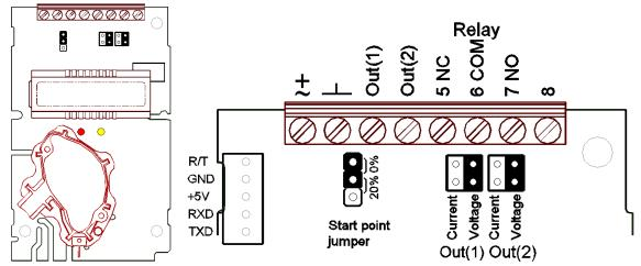
Figure 2 The aSENSE RL PCB with jumpers and terminal area enlarged at right
