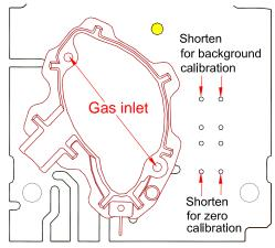
Figure 3 Holes to shorten for calibration
